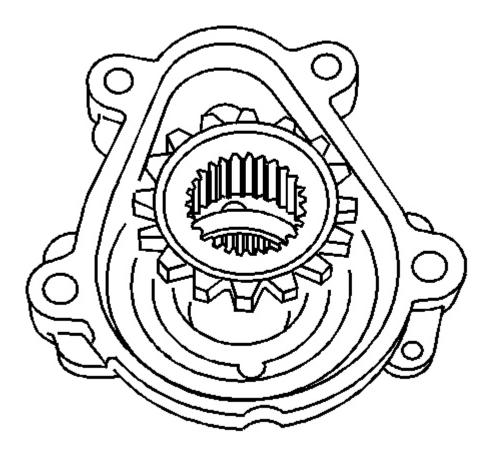
**Fig. 148: Inner Clutch Fork Gear** Courtesy of GENERAL MOTORS CORP.
