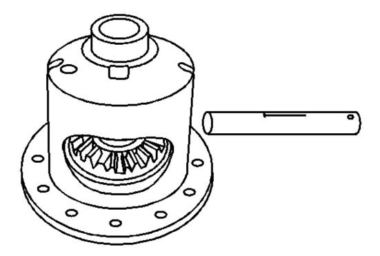
**Fig. 120: View Of Differential And Pinion Shaft** Courtesy of GENERAL MOTORS CORP.
