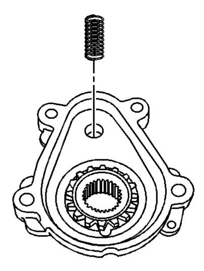
**Fig. 95: Clutch Fork Spring** Courtesy of GENERAL MOTORS CORP.
