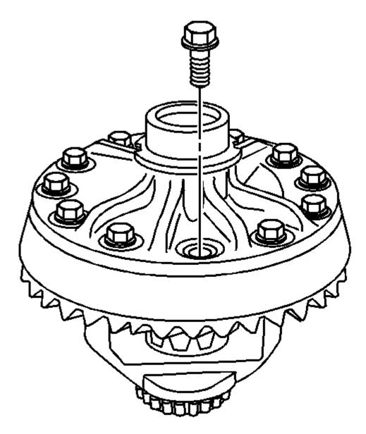
**Fig. 117: Identifying Ring Gear Bolts** Courtesy of GENERAL MOTORS CORP.
