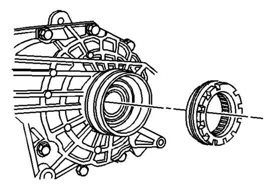
**Fig. 105: Right Side Differential Bearing Adjuster Courtesy of GENERAL MOTORS CORP.**
