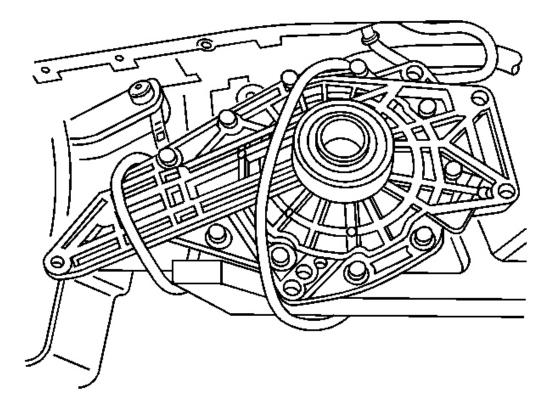
**Fig. 74: Securing Front Differential To Frame** Courtesy of GENERAL MOTORS CORP.
