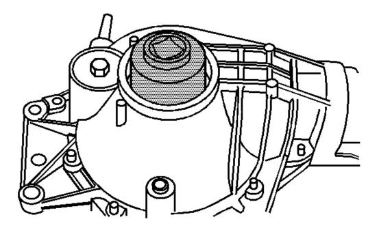
**<u>Fig. 137: Side Bearing Adjuster</u>** Courtesy of GENERAL MOTORS CORP.
