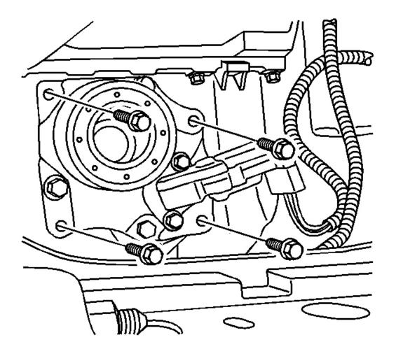
**Fig. 37: Intermediate Shaft Bearing Assembly Mounting Bolts - Front Drive Axle (S4WD)** Courtesy of GENERAL MOTORS CORP.
