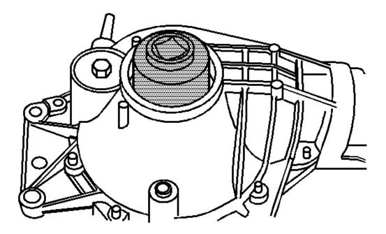
**<u>Fig. 102: Side Bearing Adjuster</u>** Courtesy of GENERAL MOTORS CORP.
