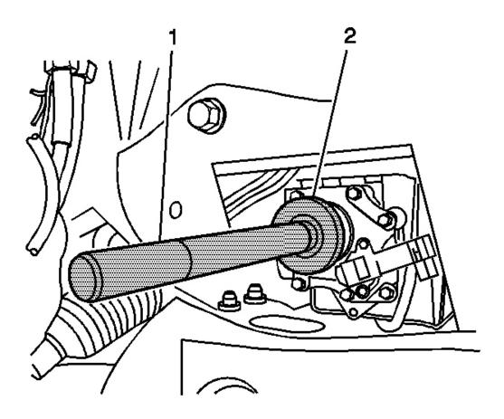
**Fig. 43: Installing Oil Seal Using Axle Seal Installer And Universal Driver Handle** Courtesy of GENERAL MOTORS CORP.
