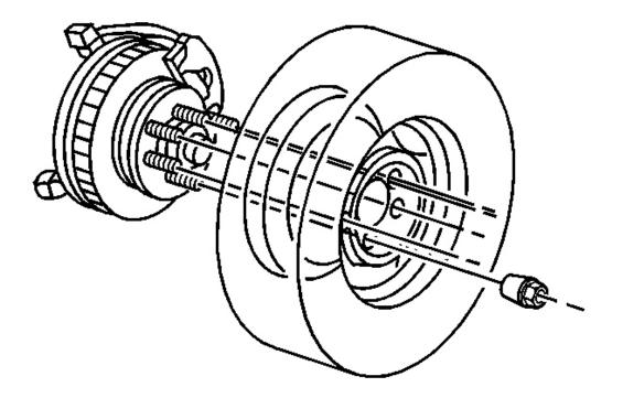
**Fig. 56: View Of Tire/Wheel Assembly, Hub Assembly & Wheel Nuts** Courtesy of GENERAL MOTORS CORP.
