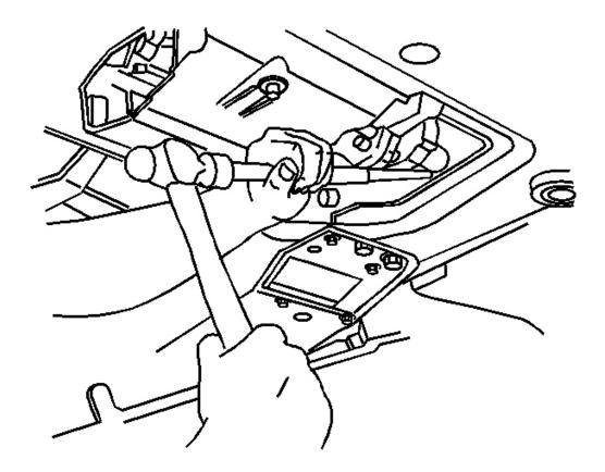
**Fig. 65: Removing Left Wheel Drive Shaft From Front Differential** Courtesy of GENERAL MOTORS CORP.
