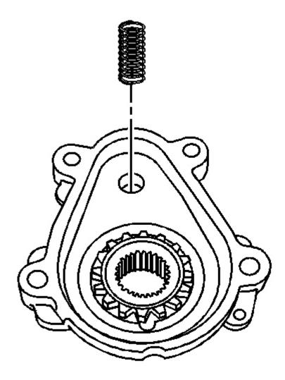
**Fig. 149: Clutch Fork Spring** Courtesy of GENERAL MOTORS CORP.
