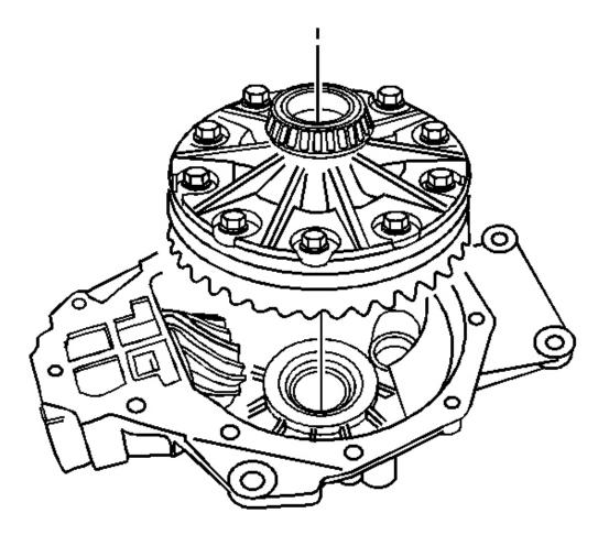
**Fig. 101: Differential Case Assembly** Courtesy of GENERAL MOTORS CORP.
