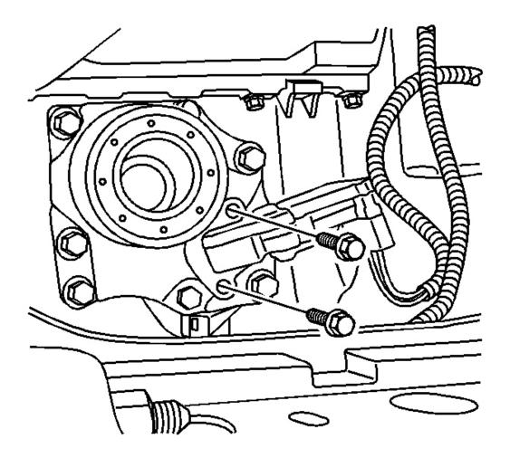
**Fig. 47: Actuator Assembly Bolts** Courtesy of GENERAL MOTORS CORP.
