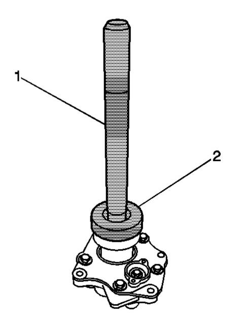
**Fig. 156:** Axle Seal Installer And Universal Driver Handle Courtesy of GENERAL MOTORS CORP.
