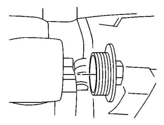
**Fig. 27: Front Axle Fill Plug** Courtesy of GENERAL MOTORS CORP.
