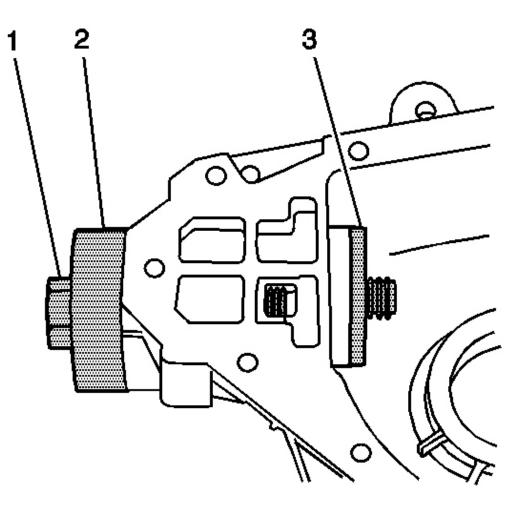
Fig. 125: J 45228-1, J 45228-2 And J 45228-5 Installed Into Pinion Bearing Cup Bore Courtesy of GENERAL MOTORS CORP.
