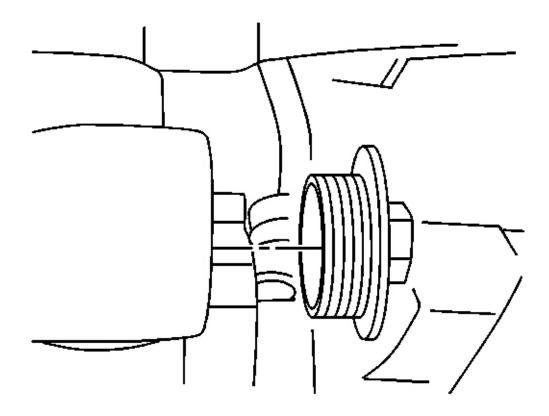
**Fig. 28: Front Axle Fill Plug** Courtesy of GENERAL MOTORS CORP.
