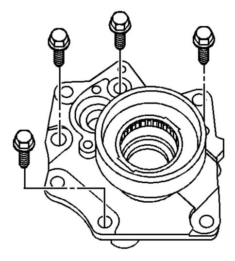
**Fig. 154: Intermediate Shaft Bearing Case Bolts Courtesy of GENERAL MOTORS CORP.**
