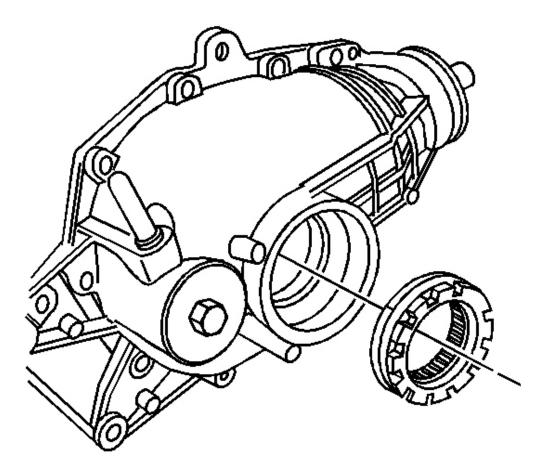
**Fig. 103: Left Side Differential Bearing Adjuster** Courtesy of GENERAL MOTORS CORP.
