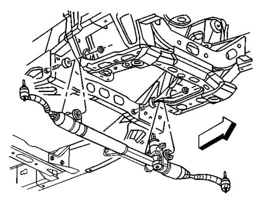
**Fig. 62: View Of Power Steering Gear & Bolts Courtesy of GENERAL MOTORS CORP.**
