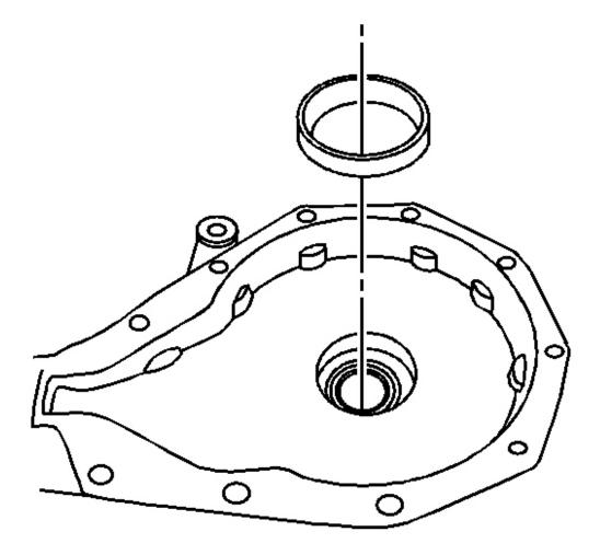
**Fig. 106: Right Side Differential Bearing Cup Courtesy of GENERAL MOTORS CORP.**
