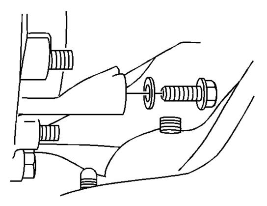
**<u>Fig. 30: Drain Plug And Washer</u>** Courtesy of GENERAL MOTORS CORP.
