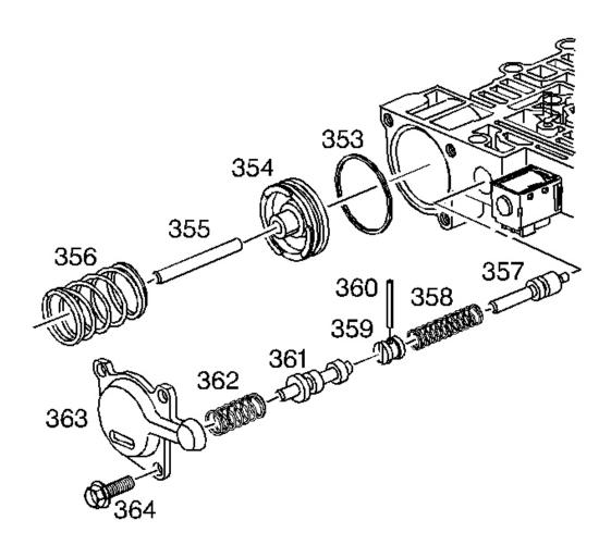
Fig. 270: Exploded View Of Forward Abuse & Low Overrun Components Courtesy of GENERAL MOTORS CORP.
