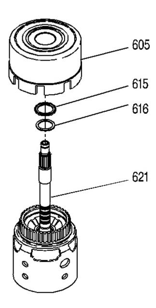
Fig. 145: View Of Stator Shaft/Selective Washer Bearing Assembly Courtesy of GENERAL MOTORS CORP.
