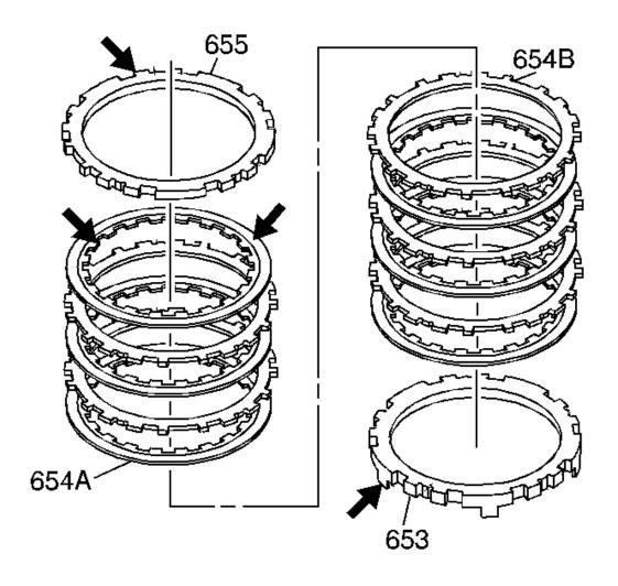
Fig. 179: View Of Inspection Areas On Clutch Apply Plates Courtesy of GENERAL MOTORS CORP.
