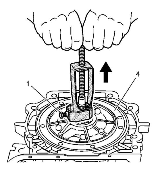
Fig. 61: Installing J 37789-A & J 39119 Courtesy of GENERAL MOTORS CORP.
