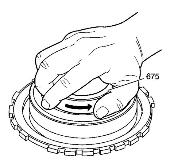
Fig. 118: Checking Low And Reverse Roller Clutch Race Rotation Courtesy of GENERAL MOTORS CORP.
