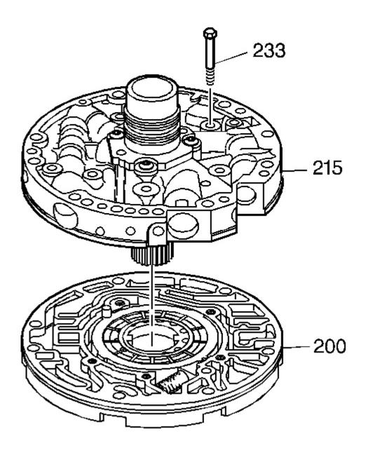
Fig. 207: Locating Pump Cover Bolts
