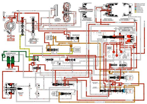
Fig. 333: Manual Second Gear Courtesy of GENERAL MOTORS CORP.
