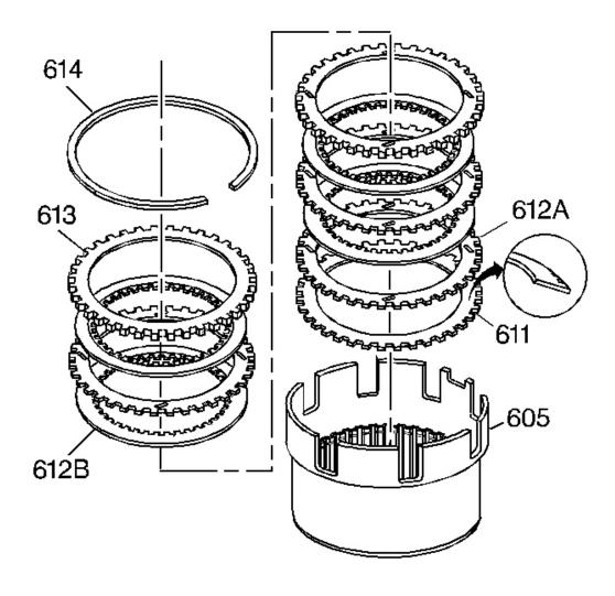
Fig. 187: Locating Reverse Input Clutch Plates Courtesy of GENERAL MOTORS CORP.
