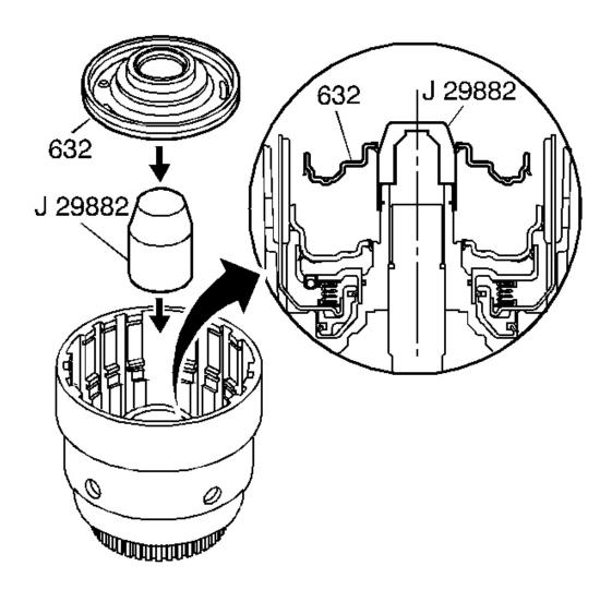
Fig. 161: Identifying Overrun Clutch Piston Courtesy of GENERAL MOTORS CORP.
