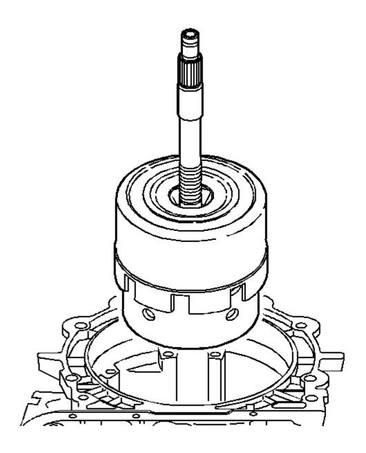
Fig. 64: Removing Input Housing And Shaft Assembly & Reverse Input Clutch Housing And Drum Assembly
