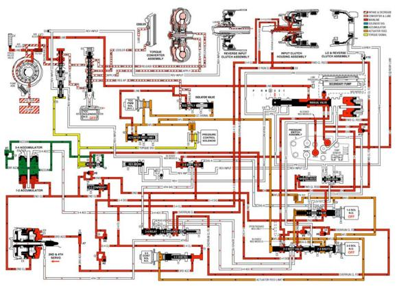
Fig. 332: Manual Third Gear Courtesy of GENERAL MOTORS CORP.
