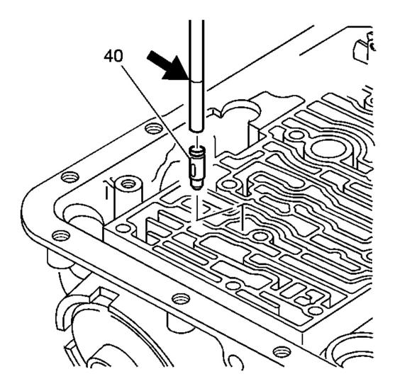
Fig. 94: Installing Third Accumulator Retainer And Ball Assembly Courtesy of GENERAL MOTORS CORP.
