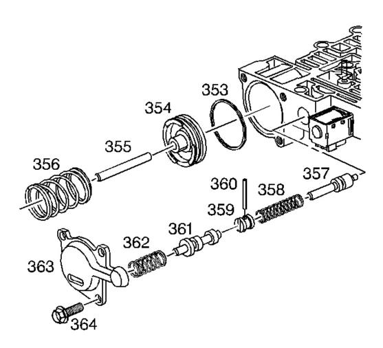
Fig. 250: Exploded View Of Forward Abuse & Low Overrun Components Courtesy of GENERAL MOTORS CORP.
