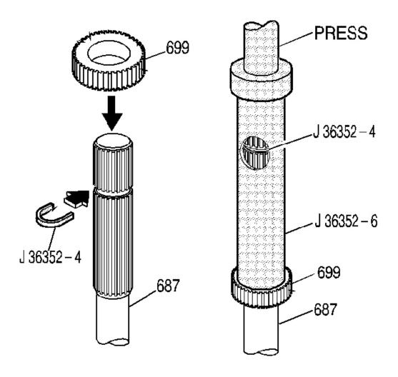
Fig. 135: Pressing Internal Speed Sensor Rotor Onto Output Shaft Courtesy of GENERAL MOTORS CORP.
