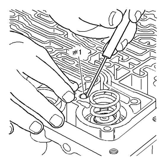
Fig. 279: Locating #1 Checkball Courtesy of GENERAL MOTORS CORP.
