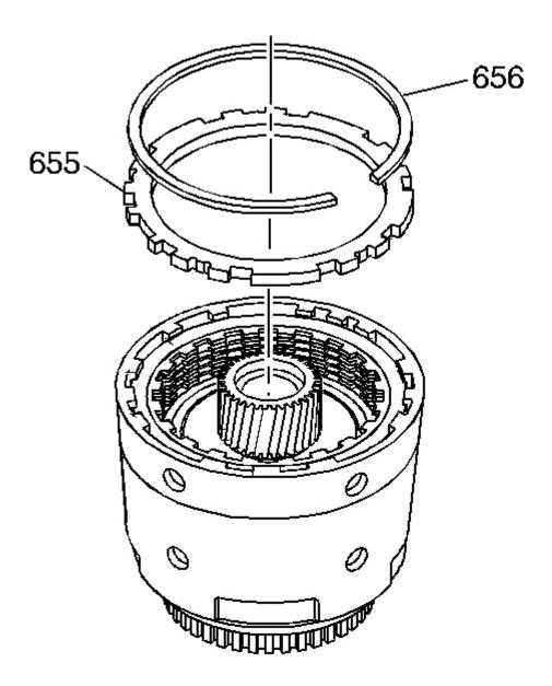
Fig. 183: Locating 3rd & 4th Clutch Selective Backing Plate & Retainer Ring Courtesy of GENERAL MOTORS CORP.
