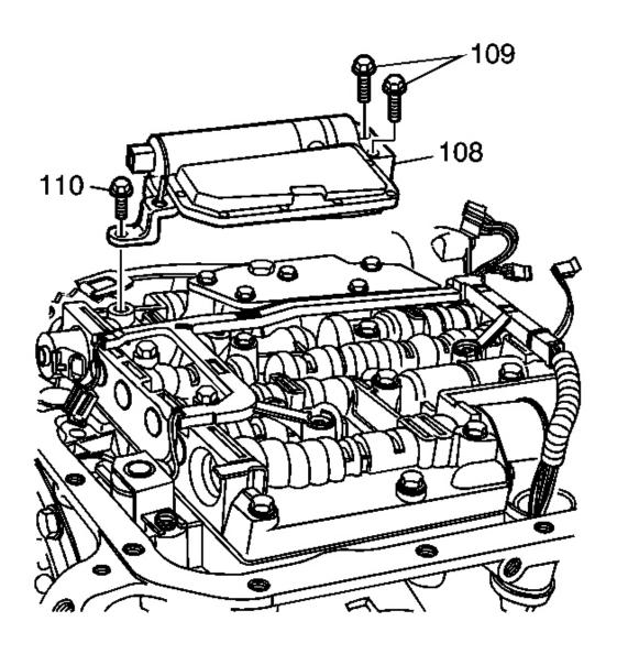
Fig. 294: Identifying Secondary Fluid Pump Courtesy of GENERAL MOTORS CORP.
