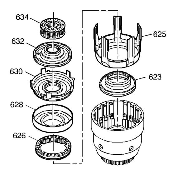
Fig. 150: Input Clutch Assembly
