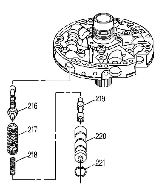
Fig. 222: View Of Reverse Boost Valve & Pressure Regulator Components
