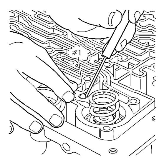
Fig. 54: Locating #1 Checkball Courtesy of GENERAL MOTORS CORP.
