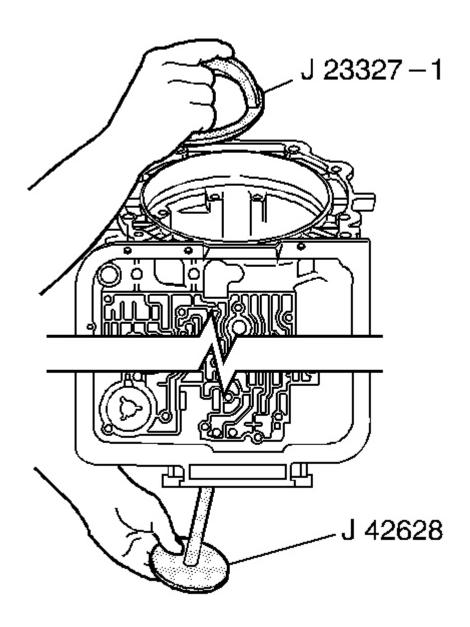
Fig. 82: Installing J 23327-1 & J 42628 Courtesy of GENERAL MOTORS CORP.
