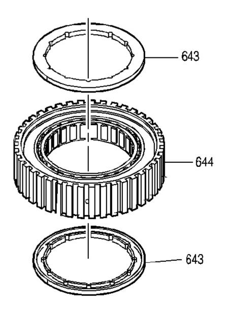
Fig. 170: View Of Sprag Assembly Retainer Rings Courtesy of GENERAL MOTORS CORP.
