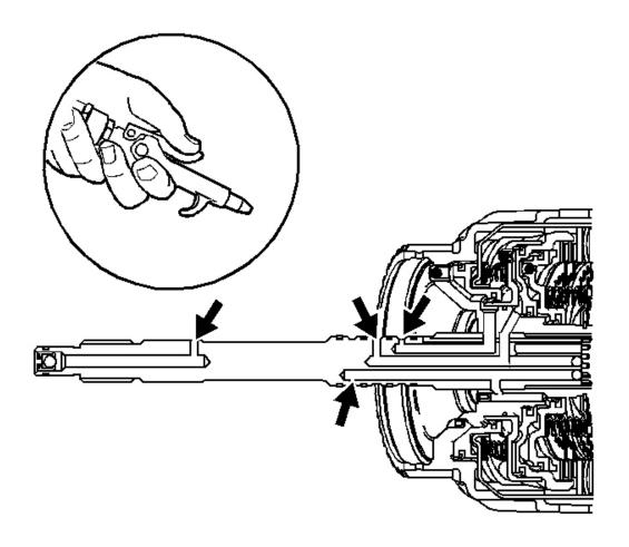
Fig. 152: Blowing Air Into Oil Feed Passages Courtesy of GENERAL MOTORS CORP.
