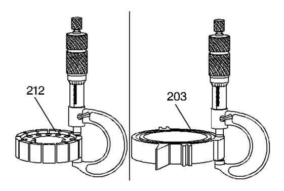
Fig. 211: Measuring Oil Pump Rotor & Slide Courtesy of GENERAL MOTORS CORP.
