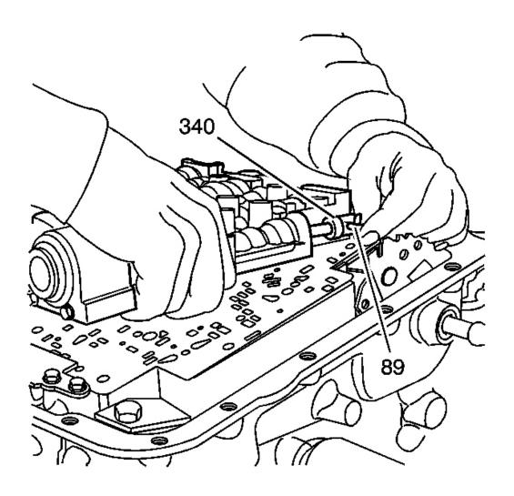
Fig. 48: Disconnecting Manual Valve Link Courtesy of GENERAL MOTORS CORP.
