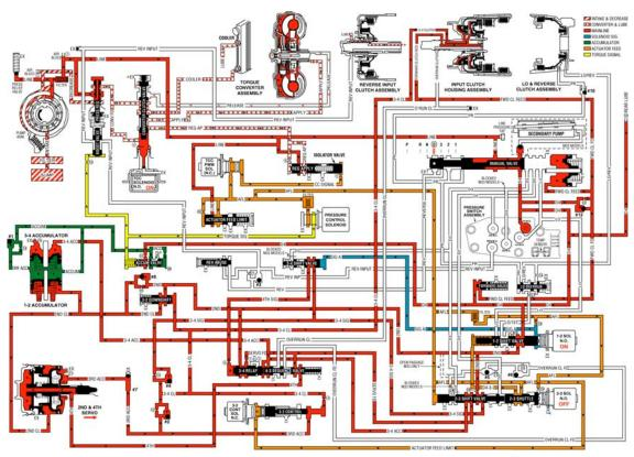
Fig. 329: Overdrive Range, Fourth Gear - TCC Applied Courtesy of GENERAL MOTORS CORP.
