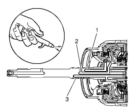
Fig. 185: Applying Air To Check Overrun Clutch Courtesy of GENERAL MOTORS CORP.
