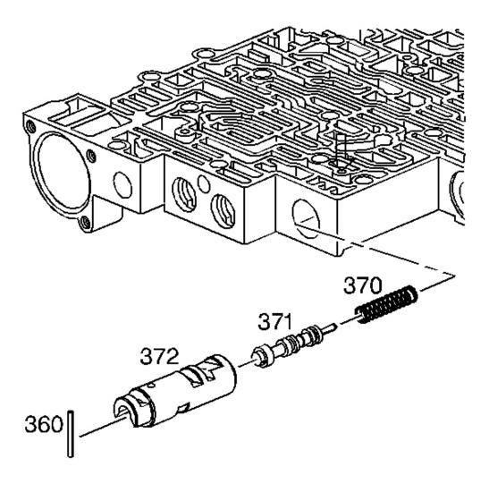
Fig. 267: View Of 1-2 Accumulator Valve & 1-2 Accumulator Valve Sleeve Courtesy of GENERAL MOTORS CORP.
