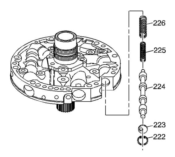
Fig. 223: Locating Converter Clutch Valve Courtesy of GENERAL MOTORS CORP.
