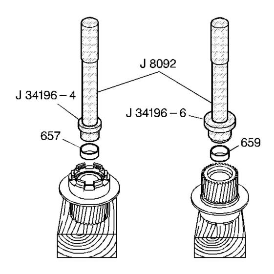
Fig. 140: Installing Input Sun Gear Front Bushing Courtesy of GENERAL MOTORS CORP.
