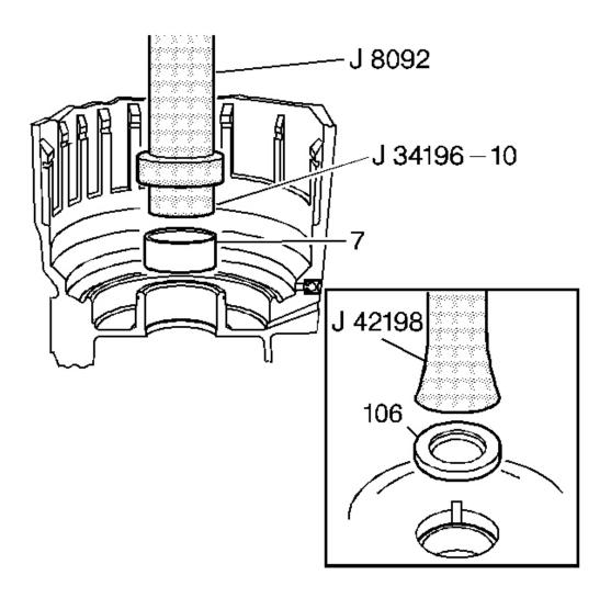
Fig. 98: View Of Case Bushing & Case Rear Oil Seal Courtesy of GENERAL MOTORS CORP.
