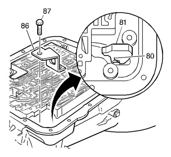
Fig. 103: Locating Parking Brake Pawl & Return Spring Courtesy of GENERAL MOTORS CORP.
