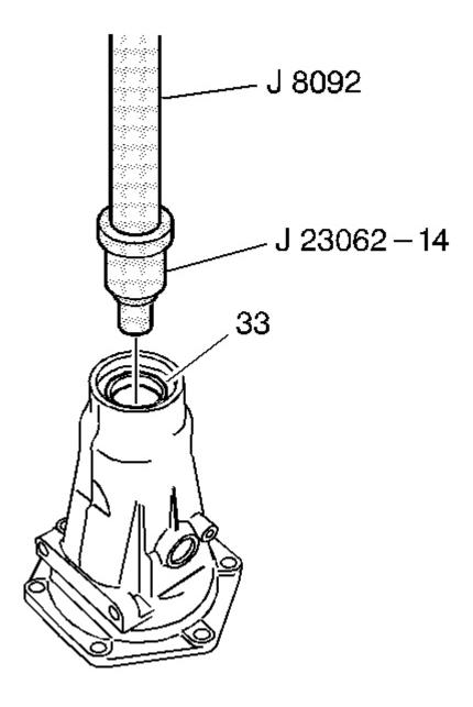
Fig. 312: Removing Case Extension Bushing Courtesy of GENERAL MOTORS CORP.
