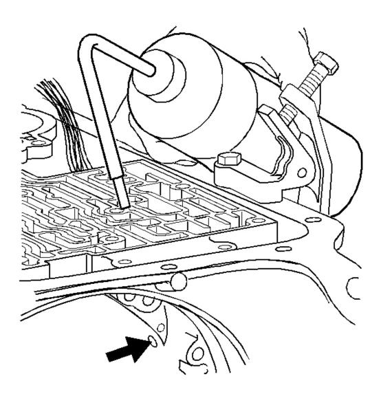
Fig. 91: Locating Small Hole In Accumulator Courtesy of GENERAL MOTORS CORP.
