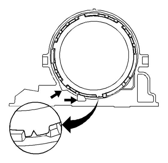
Fig. 115: Illustrating Steel Plate Spline Alignment Courtesy of GENERAL MOTORS CORP.
