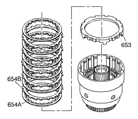
Fig. 180: Installing Clutch Apply Plates Into Input Housing Courtesy of GENERAL MOTORS CORP.
