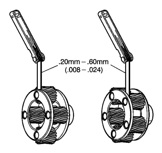
Fig. 138: Identifying Input Carrier Pinion End Play Measurements Courtesy of GENERAL MOTORS CORP.
