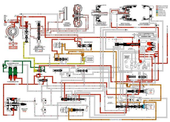
Fig. 331: Overdrive Range, 3-2 Downshift Courtesy of GENERAL MOTORS CORP.
