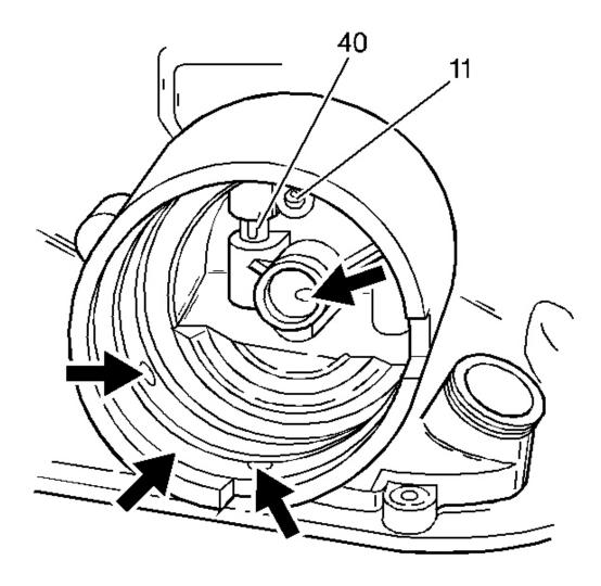
Fig. 87: Inspecting Case Assembly Components For Damage Courtesy of GENERAL MOTORS CORP.
