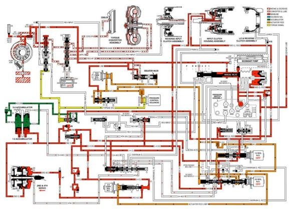
Fig. 330: Overdrive Range, 4-3 Downshift Courtesy of GENERAL MOTORS CORP.
