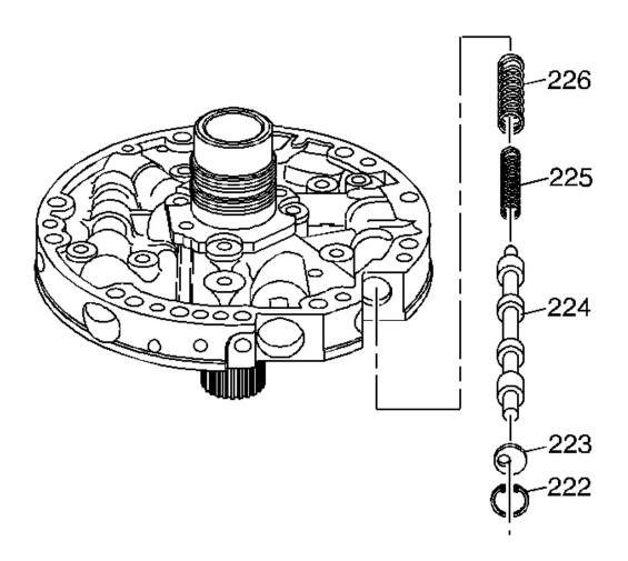
Fig. 234: Locating Converter Clutch Valve Courtesy of GENERAL MOTORS CORP.
