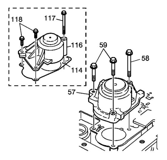
Fig. 282: Installing 1-2 Accumulator Housing Bolts Courtesy of GENERAL MOTORS CORP.
