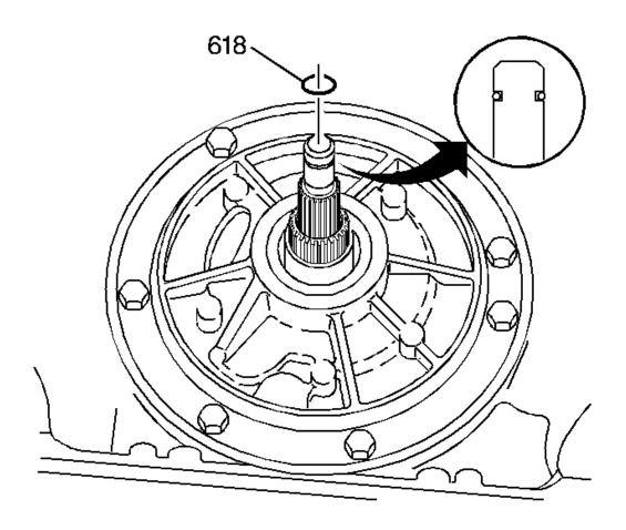
Fig. 55: Identifying Turbine Shaft O-Ring Courtesy of GENERAL MOTORS CORP.
