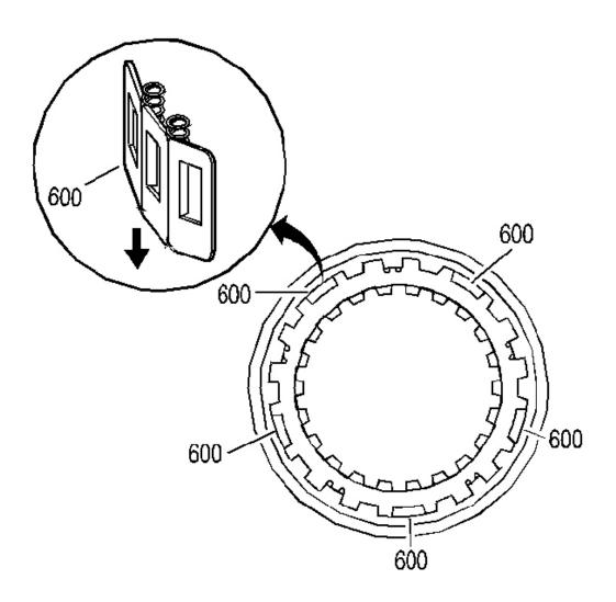
Fig. 182: Identifying 3-4 Clutch Boost Spring Assemblies Courtesy of GENERAL MOTORS CORP.
