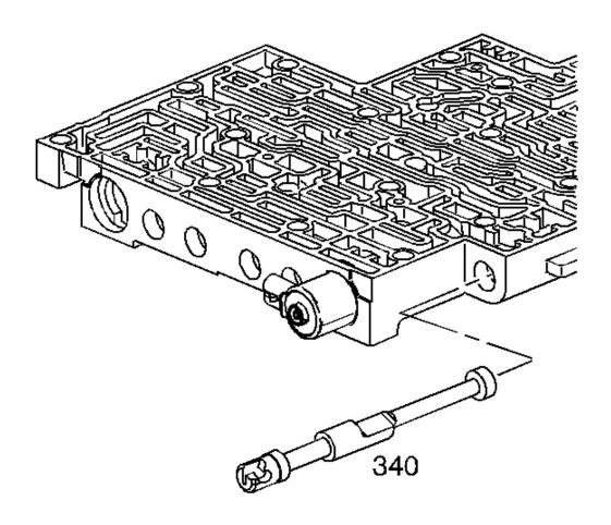
Fig. 249: View Of Manual Valve Courtesy of GENERAL MOTORS CORP.
