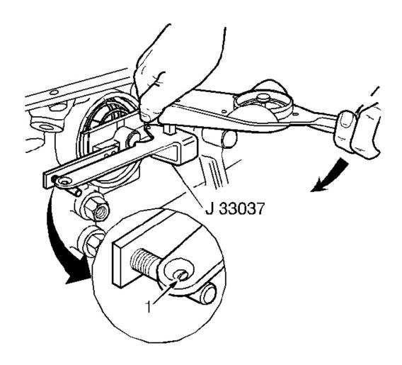
Fig. 32: Identifying Gage Slot Courtesy of GENERAL MOTORS CORP.
