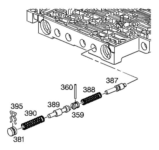
Fig. 256: View Of Reverse Abuse Valve & 3-2 Downshift Valve Courtesy of GENERAL MOTORS CORP.
