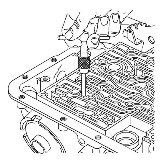
Fig. 92: Extracting Third Accumulator Retainer And Ball Assembly Courtesy of GENERAL MOTORS CORP.
