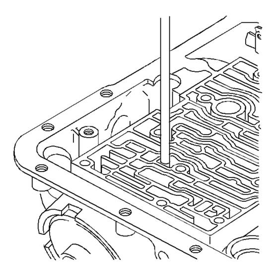
Fig. 95: Checking Third Accumulator Retainer And Ball Assembly Alignment Courtesy of GENERAL MOTORS CORP.
