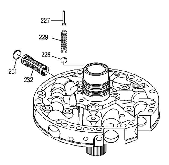
Fig. 233: View Of Oil Pump Cover Screen Courtesy of GENERAL MOTORS CORP.
