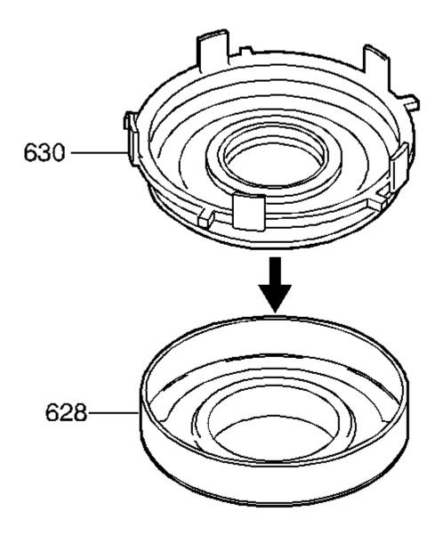
Fig. 157: Installing Forward Clutch Piston Courtesy of GENERAL MOTORS CORP.
