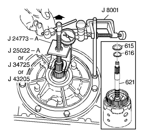
Fig. 246: Checking End Play With J 8001 Courtesy of GENERAL MOTORS CORP.
