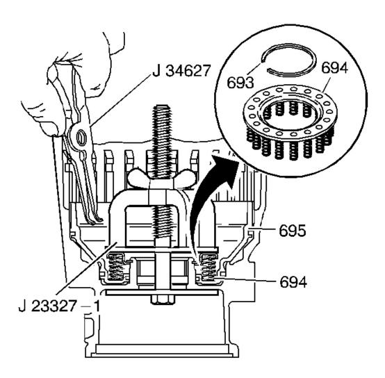
Fig. 83: View Of Low And Reverse Clutch Spring Assembly & Retainer Ring Courtesy of GENERAL MOTORS CORP.
