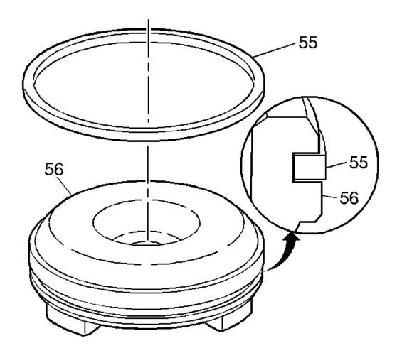
Fig. 275: Inspecting 1-2 Accumulator Piston Courtesy of GENERAL MOTORS CORP.
