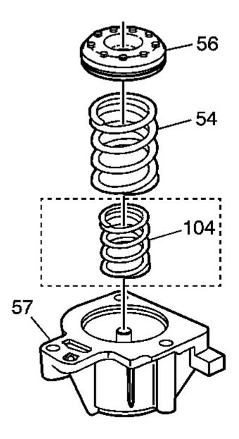
Fig. 277: View Of 1-2 Inner & Outer Springs Courtesy of GENERAL MOTORS CORP.
