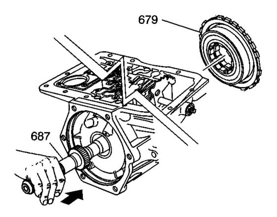
Fig. 73: View Of Low And Reverse Clutch Support Courtesy of GENERAL MOTORS CORP.
