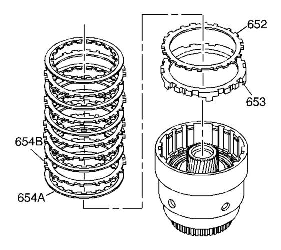
Fig. 181: Illustrating Clutch Plate Assembly
