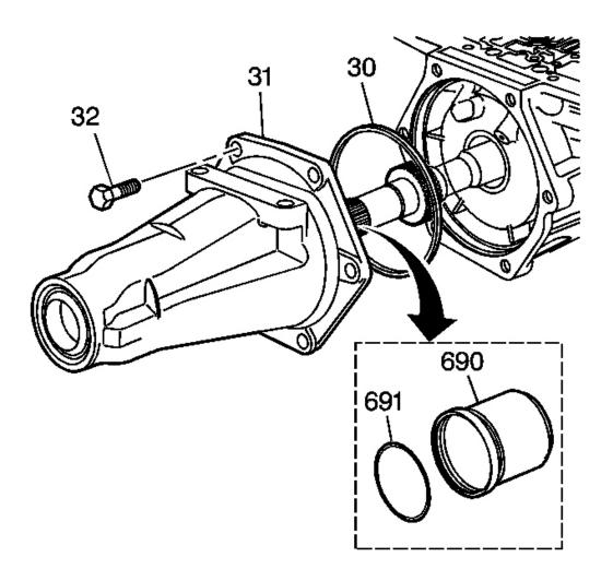
Fig. 34: Identifying Output Shaft Components Courtesy of GENERAL MOTORS CORP.
