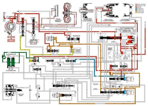
Fig. 326: Overdrive Range, First Gear Courtesy of GENERAL MOTORS CORP.
