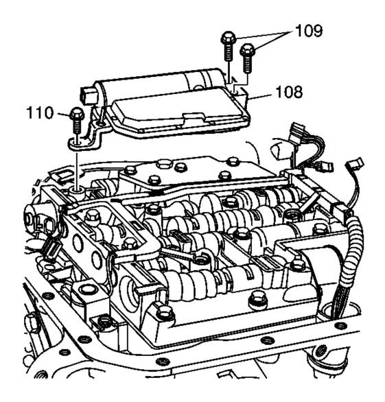
Fig. 40: Identifying Secondary Fluid Pump Courtesy of GENERAL MOTORS CORP.
