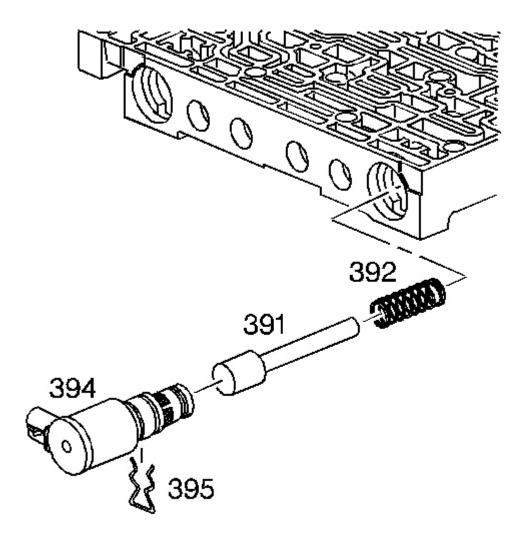
Fig. 265: Identifying 3-2 Control Valve & 3-2 Control Solenoid Courtesy of GENERAL MOTORS CORP.
