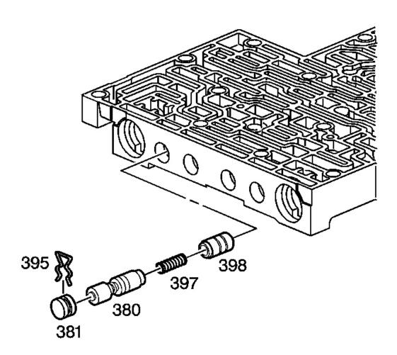
Fig. 261: Identifying Isolator Valve & Regulator Apply Valve Courtesy of GENERAL MOTORS CORP.
