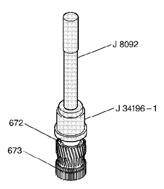
Fig. 123: Removing Reaction Sun Bushing From Reaction Sun Gear Courtesy of GENERAL MOTORS CORP.
