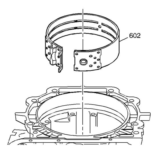
Fig. 65: View Of 2-4 Band Assembly Courtesy of GENERAL MOTORS CORP.
