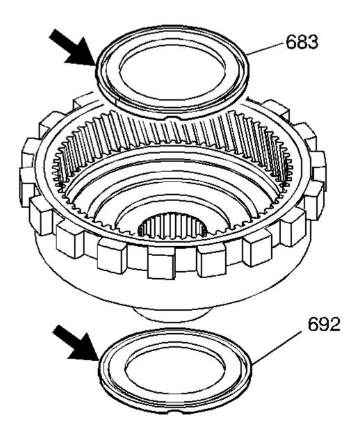
Fig. 105: Inspecting Areas Of Reaction Carrier/Support Thrust Bearing Assembly Courtesy of GENERAL MOTORS CORP.
