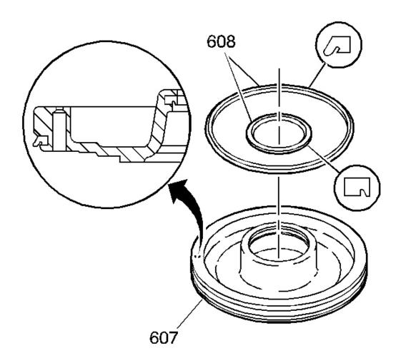
Fig. 195: Locating Inspection Areas On Reverse Input Clutch Piston Courtesy of GENERAL MOTORS CORP.
