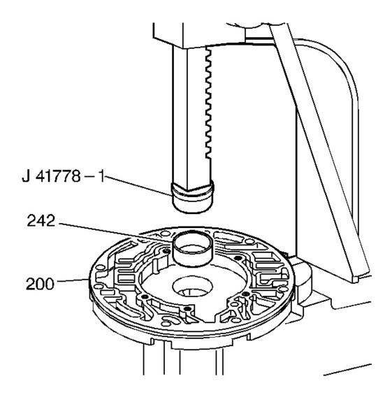
Fig. 215: Pressing In Pump Body Bushing Courtesy of GENERAL MOTORS CORP.
