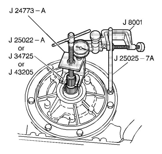
Fig. 58: Installing J 25025-7A With J 8001 Courtesy of GENERAL MOTORS CORP.
