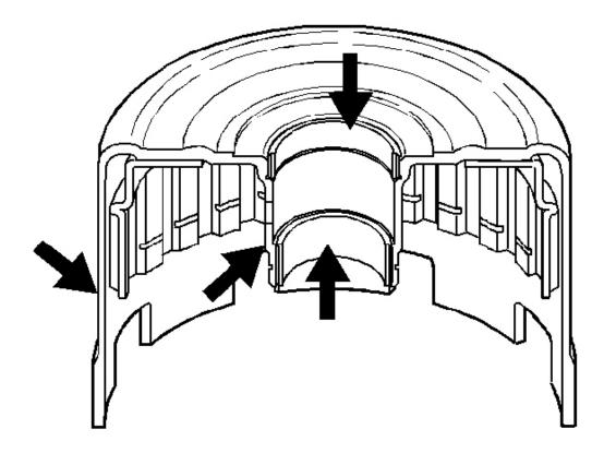
Fig. 190: Inspection Areas On Reverse Input Clutch Housing & Drum Assembly Courtesy of GENERAL MOTORS CORP.
