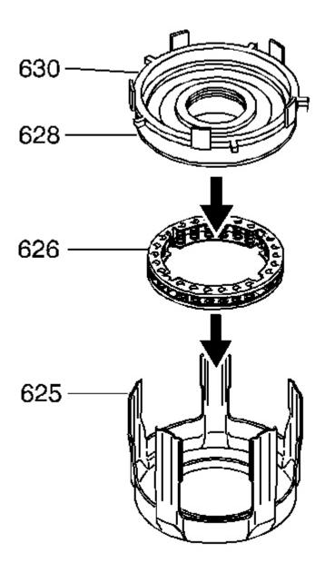
Fig. 158: Locating 3rd & 4th Spring Assembly Courtesy of GENERAL MOTORS CORP.
