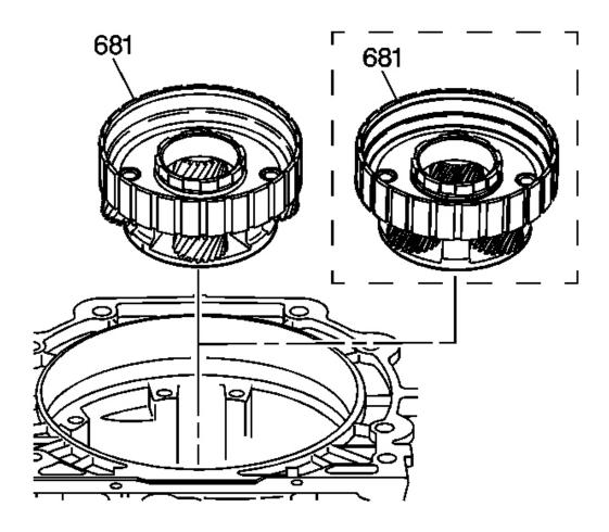
Fig. 76: Identifying Reaction Carrier Assembly Courtesy of GENERAL MOTORS CORP.
