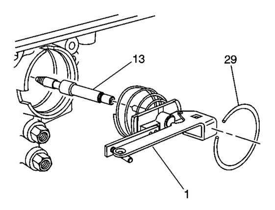
Fig. 301: Locating Servo Cover Retaining Ring Courtesy of GENERAL MOTORS CORP.
