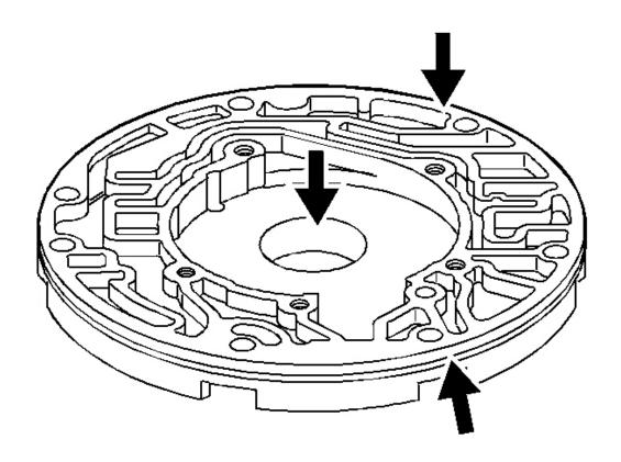
Fig. 212: Identifying Oil Pump Body Inspection Areas Courtesy of GENERAL MOTORS CORP.
