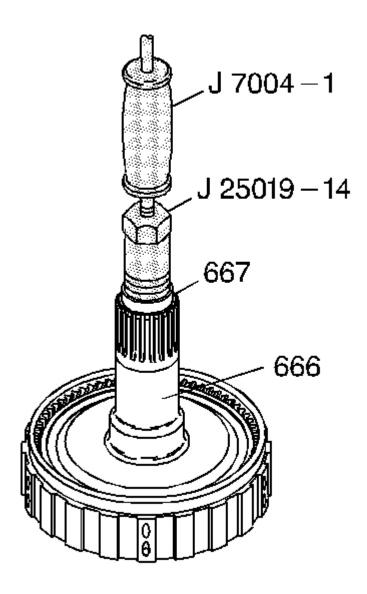
Fig. 129: Using J 25019-14 & J 25019-14 To Remove Reaction Carrier Shaft Rear Bushing Courtesy of GENERAL MOTORS CORP.
