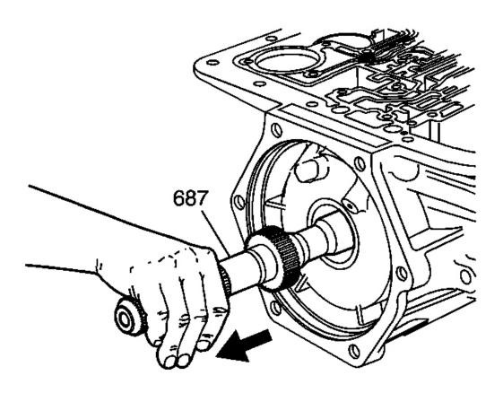
Fig. 74: Locating Output Shaft
