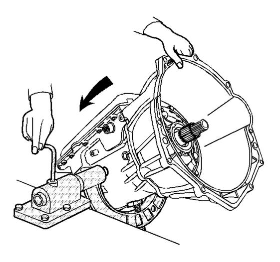
Fig. 24: Draining Transmission Oil Courtesy of GENERAL MOTORS CORP.
