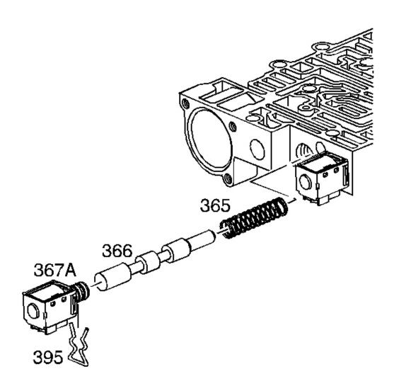
Fig. 269: Locating 1-2 Shift Valve & Solenoid Components Courtesy of GENERAL MOTORS CORP.
