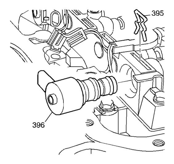
Fig. 42: Removing TCC/PWM Solenoid & Clip Courtesy of GENERAL MOTORS CORP.
