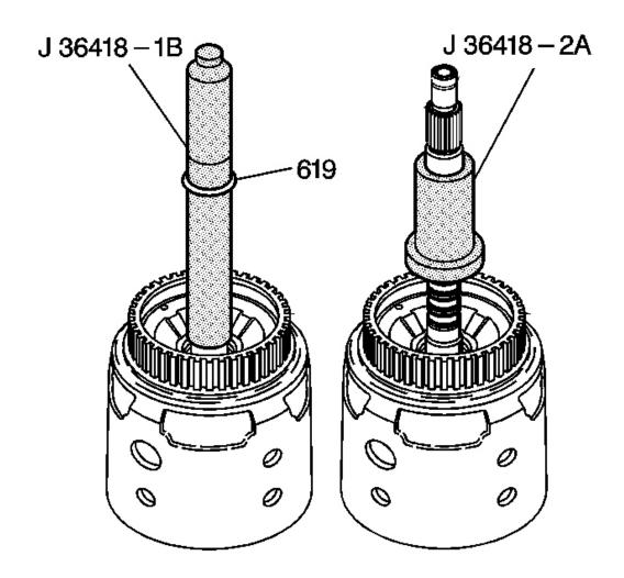
Fig. 186: Identifying J 36418-1B & J 36418-2A Courtesy of GENERAL MOTORS CORP.
