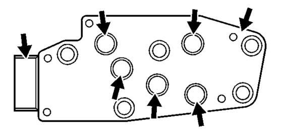
Fig. 287: Inspection Areas On Transmission Fluid Pressure (TFP) Manual Valve Position Switch
