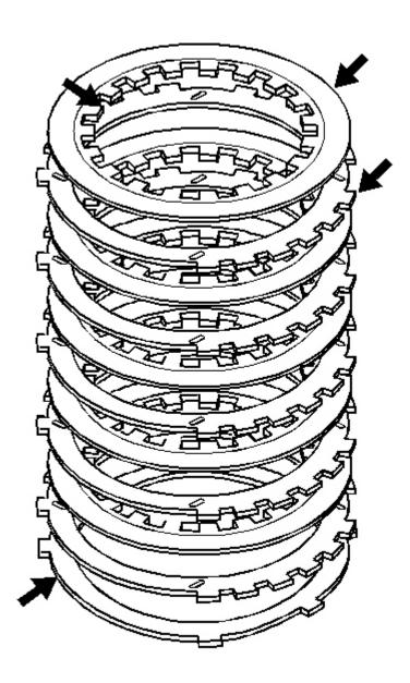
Fig. 111: Locating Inspection Areas On Low And Reverse Clutch Plates Courtesy of GENERAL MOTORS CORP.
