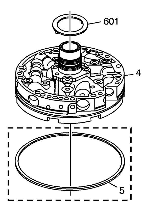
Fig. 206: View Of Pump To Drum Thrust Washer
