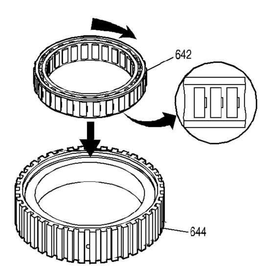
Fig. 171: Forward Sprag Assembly Courtesy of GENERAL MOTORS CORP.
