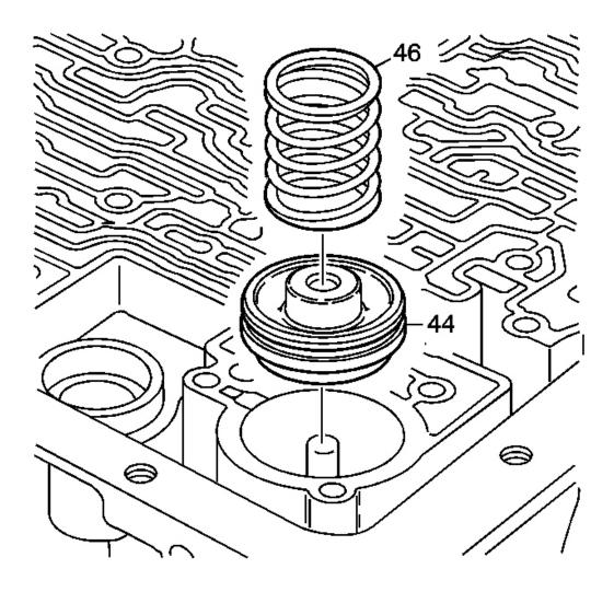
Fig. 273: View Of 3-4 Accumulator Piston & Seal Assembly Courtesy of GENERAL MOTORS CORP.
