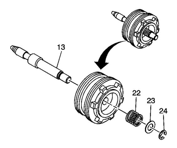
Fig. 30: 2-4 Servo Assembly Courtesy of GENERAL MOTORS CORP.
