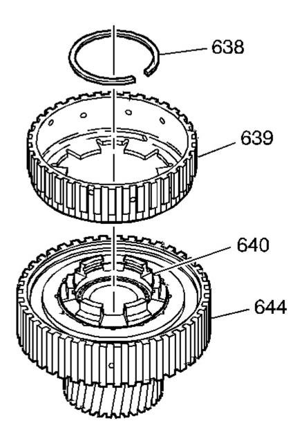
Fig. 174: Locating Overrun Clutch Hub Courtesy of GENERAL MOTORS CORP.
