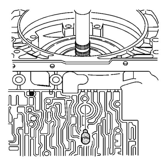
Fig. 205: Identifying Band Anchor Pin Courtesy of GENERAL MOTORS CORP.
