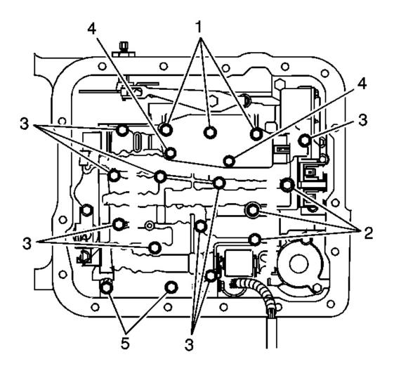
Fig. 290: Locating Valve Body Bolts
