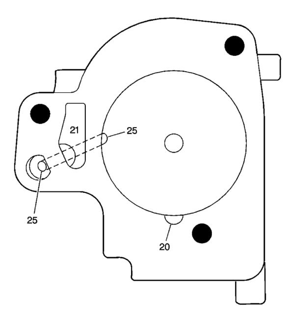
Fig. 345: 1-2 Accumulator Cover Fluid Passages Courtesy of GENERAL MOTORS CORP.
