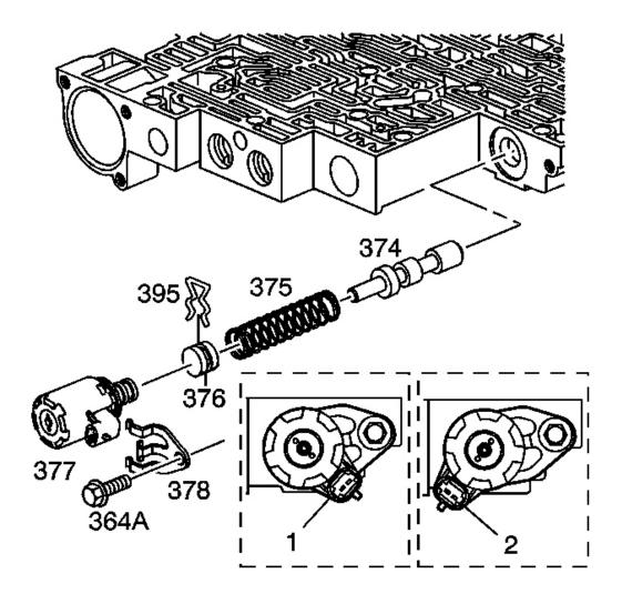
Fig. 254: View Of Pressure Control Solenoid & Components Courtesy of GENERAL MOTORS CORP.
