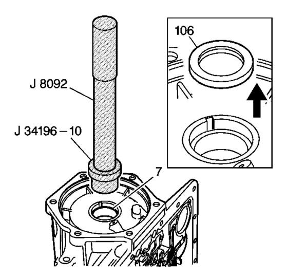
Fig. 97: Identifying Case Rear Oil Seal & Case Bushing Courtesy of GENERAL MOTORS CORP.
