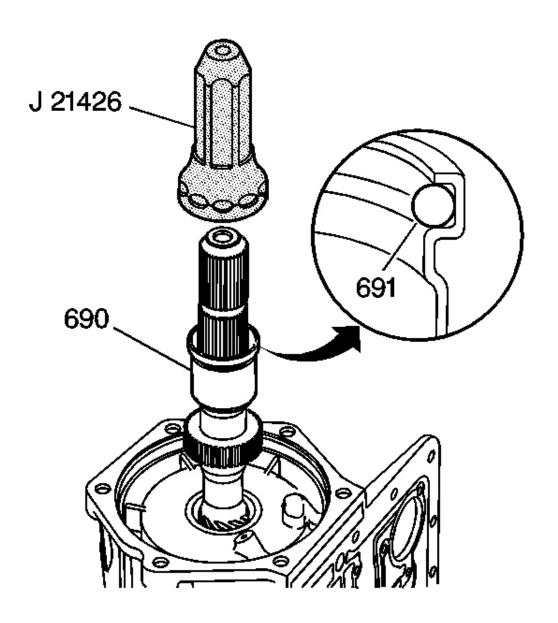
Fig. 314: Cross Sectional View Of Output Shaft Seal Courtesy of GENERAL MOTORS CORP.
