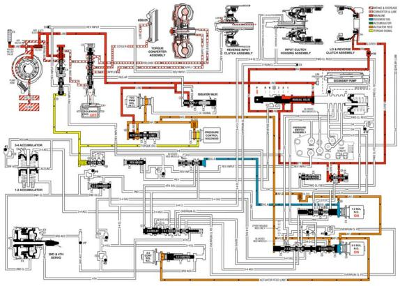
Fig. 323: Park - Engine Running Courtesy of GENERAL MOTORS CORP.
