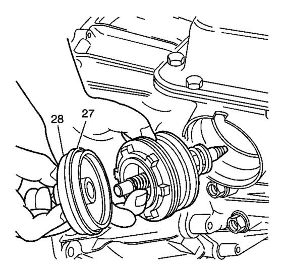
Fig. 29: View Of 2-4 Servo Assembly Courtesy of GENERAL MOTORS CORP.
