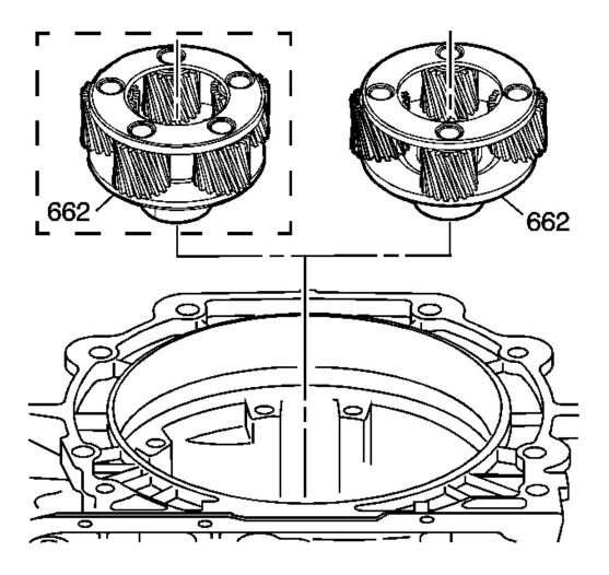
Fig. 142: Locating Input Carrier Assembly Courtesy of GENERAL MOTORS CORP.
