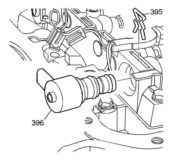
Fig. 291: Locating TCC PWM Solenoid Valve Courtesy of GENERAL MOTORS CORP.
