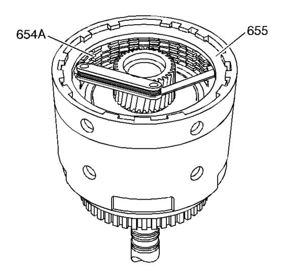
Fig. 184: Checking 3rd & 4th Clutch Plate Travel Courtesy of GENERAL MOTORS CORP.
