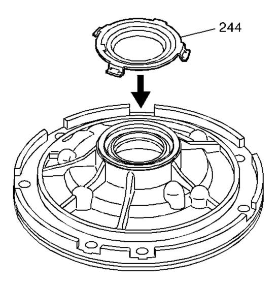
Fig. 218: Installing Front Helix Retainer Courtesy of GENERAL MOTORS CORP.
