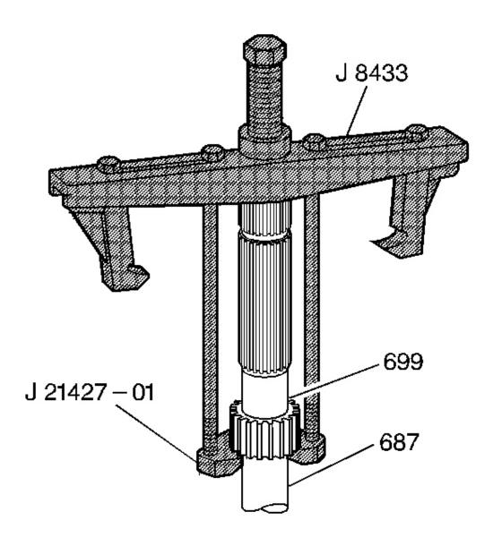
Fig. 134: Using J 8433 & J 21427-01 To Remove Internal Speed Sensor Rotor Courtesy of GENERAL MOTORS CORP.
