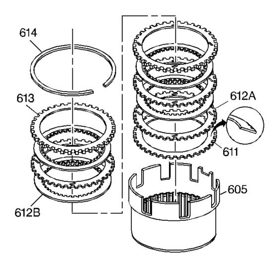
Fig. 200: Exploded View Of Reverse Input Clutch Plates Courtesy of GENERAL MOTORS CORP.
