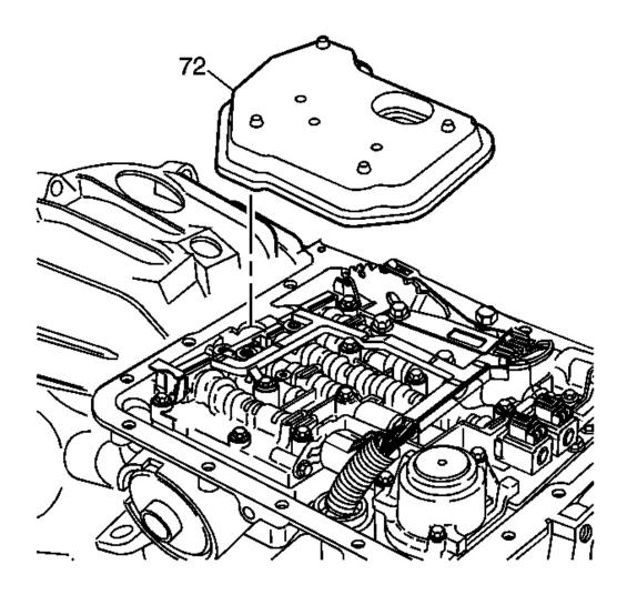
Fig. 37: Identifying Transmission Oil Filter Assembly Courtesy of GENERAL MOTORS CORP.
