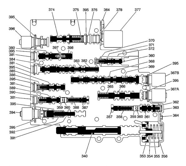
Fig. 18: Identifying Transmission Valve Body Components Courtesy of GENERAL MOTORS CORP.
