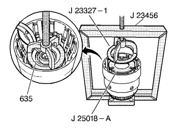
Fig. 149: Installing J 23327-1 & J 25018-A Courtesy of GENERAL MOTORS CORP.
