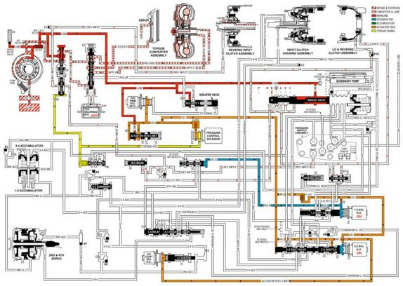
Fig. 325: Neutral - Engine Running Courtesy of GENERAL MOTORS CORP.
