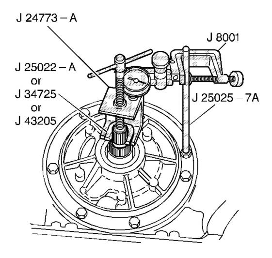
Fig. 245: Installing J 25025-7A With J 8001 Courtesy of GENERAL MOTORS CORP.
