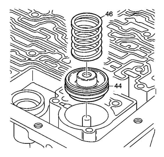
Fig. 53: View Of 3-4 Accumulator Piston & Seal Assembly Courtesy of GENERAL MOTORS CORP.
