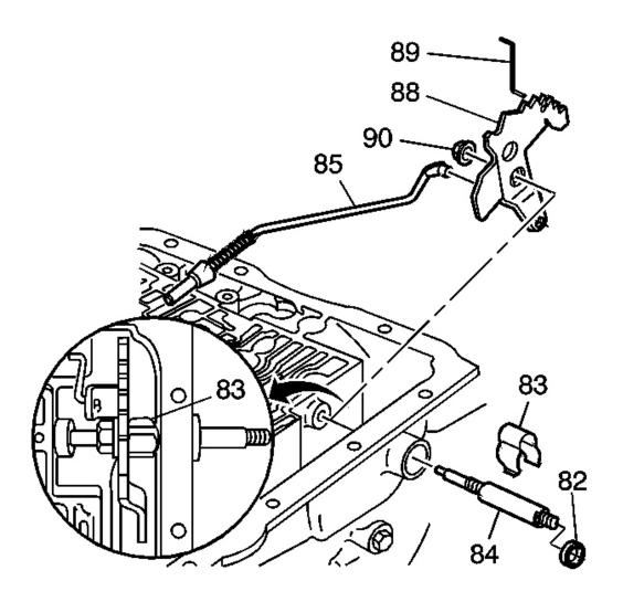
Fig. 79: Inspecting Inner Manual Linkage Courtesy of GENERAL MOTORS CORP.
