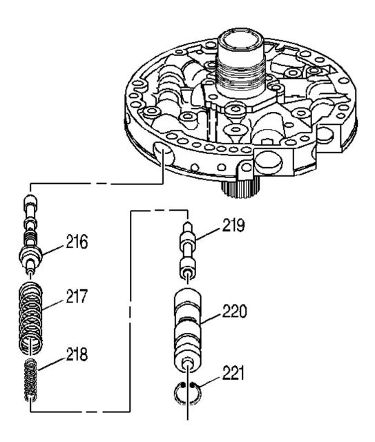
Fig. 235: View Of Pressure Regulator Valve Courtesy of GENERAL MOTORS CORP.
