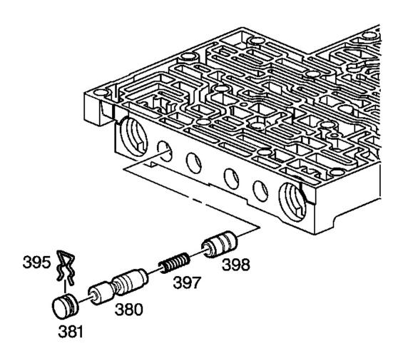
Fig. 258: Identifying Isolator Valve & Regulator Apply Valve Courtesy of GENERAL MOTORS CORP.
