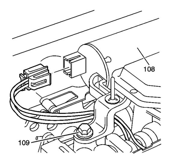
Fig. 39: Locating Secondary Fluid Pump Electrical Connector & Retaining Bolts Courtesy of GENERAL MOTORS CORP.
