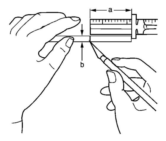
Fig. 93: Scribing Mark On Rod For Gaging Proper Depth Of Third Accumulator Retainer And Ball Assembly
