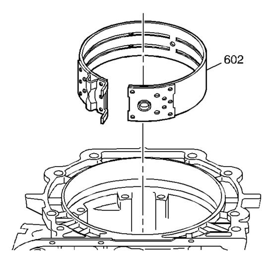
Fig. 204: View Of 2-4 Band Assembly Courtesy of GENERAL MOTORS CORP.
