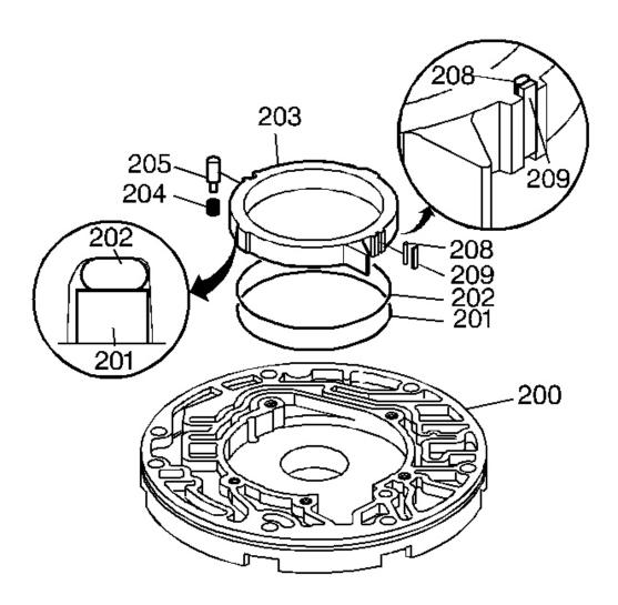
Fig. 219: Identifying Pump Slide Components Courtesy of GENERAL MOTORS CORP.
