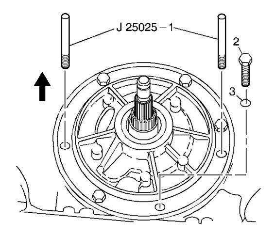
Fig. 241: View Of J 25025-1 Courtesy of GENERAL MOTORS CORP.
