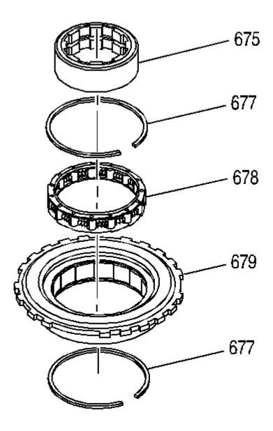
Fig. 116: Low and Reverse Clutch Support Components Courtesy of GENERAL MOTORS CORP.
