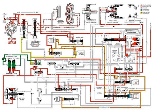
Fig. 327: Overdrive Range, Second Gear Courtesy of GENERAL MOTORS CORP.
