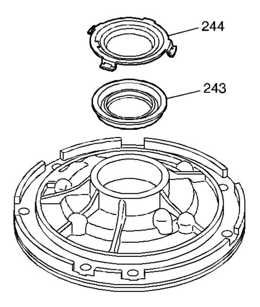
Fig. 213: Locating Front Helix Retainer & Oil Seal Assembly Courtesy of GENERAL MOTORS CORP.
