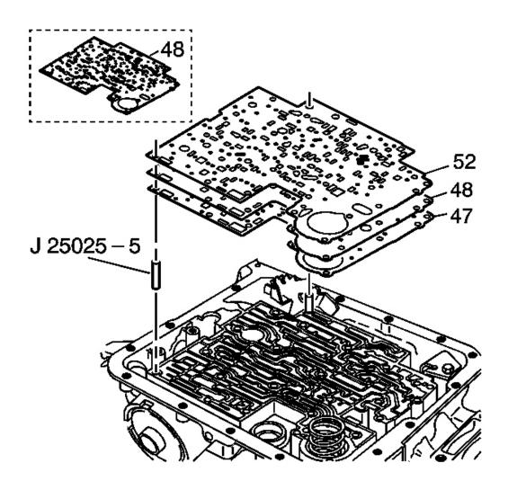
Fig. 280: Using J 25025-5 To Install Spacer Plate Courtesy of GENERAL MOTORS CORP.
