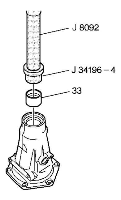
Fig. 313: Installing Case Extension Bushing Courtesy of GENERAL MOTORS CORP.
