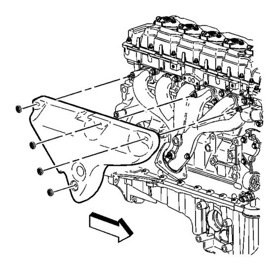
**Fig. 54: View Of Exhaust Manifold Heat Shield & Nuts Courtesy of GENERAL MOTORS CORP.**
