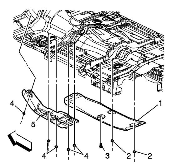
Fig. 61: View Of Catalytic Converter Heat Shields & Nuts
