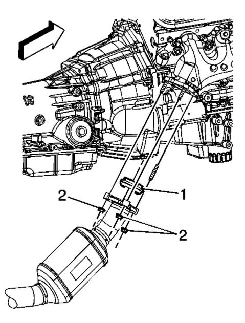
Fig. 34: View Of Exhaust Manifold, Catalytic Converter, Sealing Ring & Nuts Courtesy of GENERAL MOTORS CORP.
