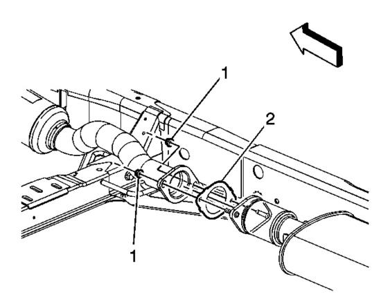
Fig. 20: View Of Catalytic Converter, Muffler, Gasket & Nuts Courtesy of GENERAL MOTORS CORP.
